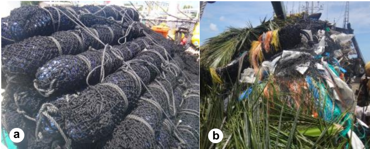
Figure 3. (a) Stack of dFAD floats built with a line of 6–8 corks covered by a sheet of plastic and wrapped in 4–5 inches netting, (b) piled up dFAD tail materials showing purse seine netting, palm leaves, white salt bags and colored attractor strips. Photos taken at port of Majuro (Marshall Islands, WCPO) in 2017.
