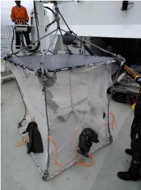
Figure 7. Short tailed FAD design, commonly known as “cage FAD”, widely used currently in the Indian Ocean.
