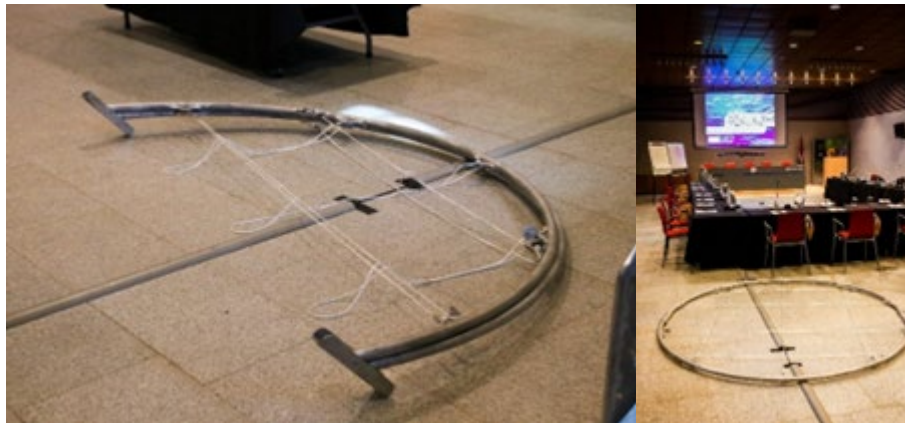
Figure 8 - Round lightweight mobulid sorting grid with hinges for folding, in its folded (left) and extended (right) formats.
