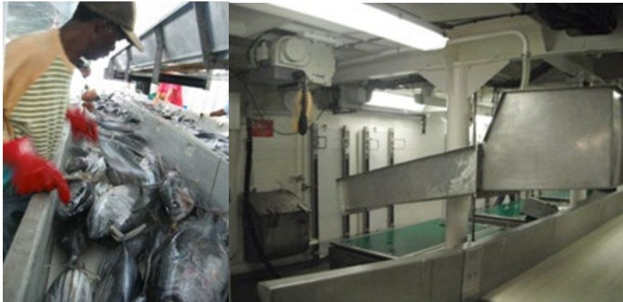
Figure 10 - Lower deck double conveyor belt for bycatch release (left) and closed gutter on the side of the lower deck wall (right).
