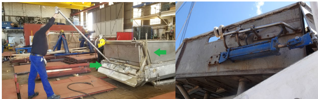
Figure 23 - Mobile hopper door stop mechanisms: manual (left) and hydraulic (right).
