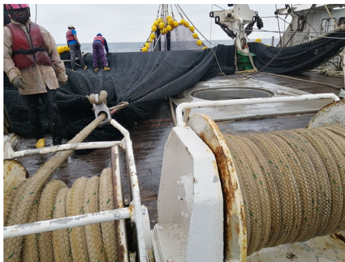
Figure 18 - A view showing the two chokers and net occupying a large proportion of the working deck during the formation of the sack.
