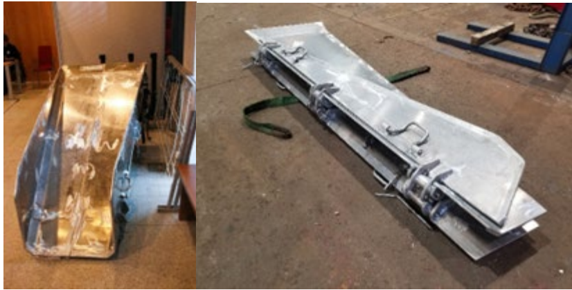
Figure 9 - Foldable bycatch release ramp (left) and ramp folded for storage (right).
