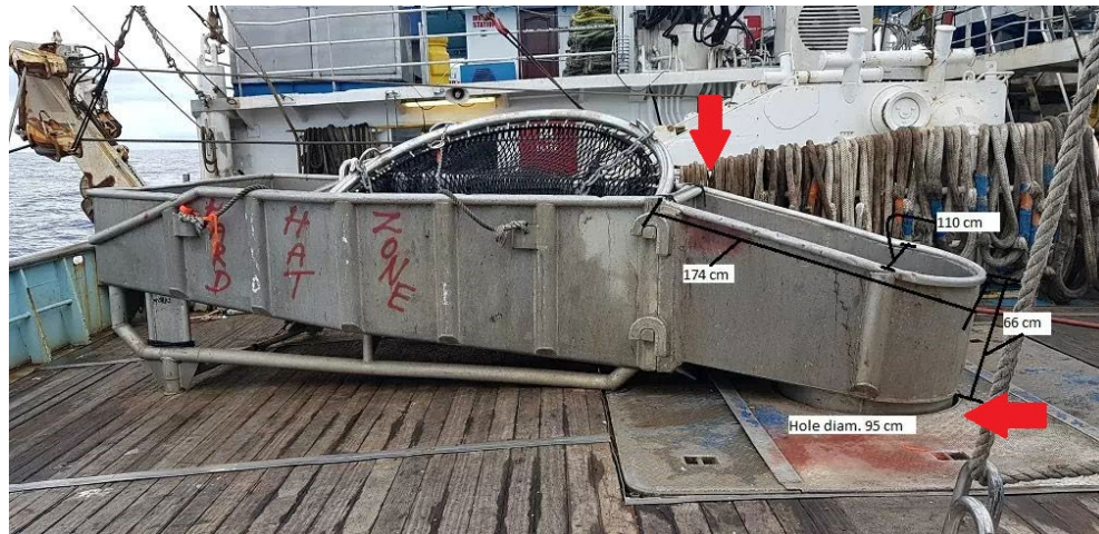
Figure 25 - Hopper with a double stop door system in the middle and at the base (red arrows).
