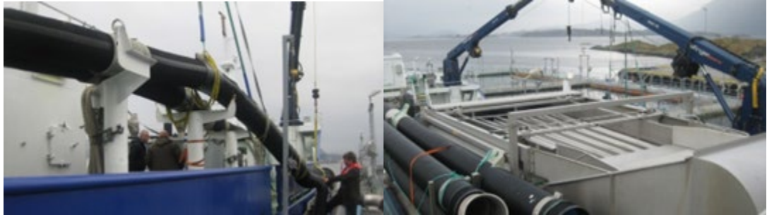
Figure 31 - Vacuum pump hoses and classification systems on the deck of well-boats for live transport of salmon in Norway.
