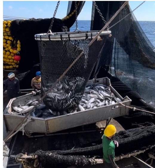
Figure 3. Some vessels use a hopper to discharge the catch and perform preliminary sorting before the fish pass through the unloading hatch into the fish wells. The use of a hopper facilitates improved release of non-target species from the upper deck. Manta sorting grids are compatible with hoppers. Photo: Melissa Cronin, Pacific Princess
