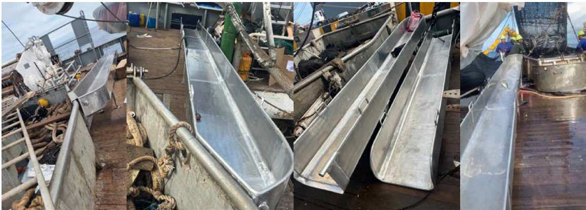
Figure 2. A release ramp system integrated with a hopper. Photos: Cape Ferrat and ISSF
