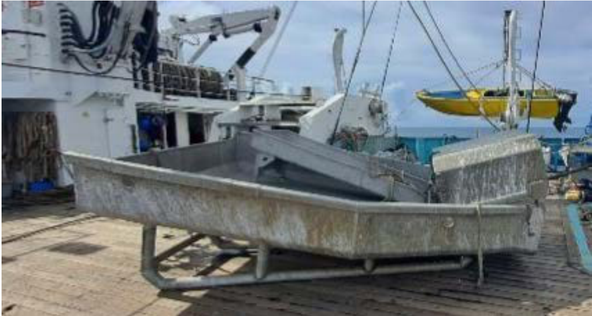
Figure 4. Release ramp stored inside the hopper tray. Photo: AZTI
