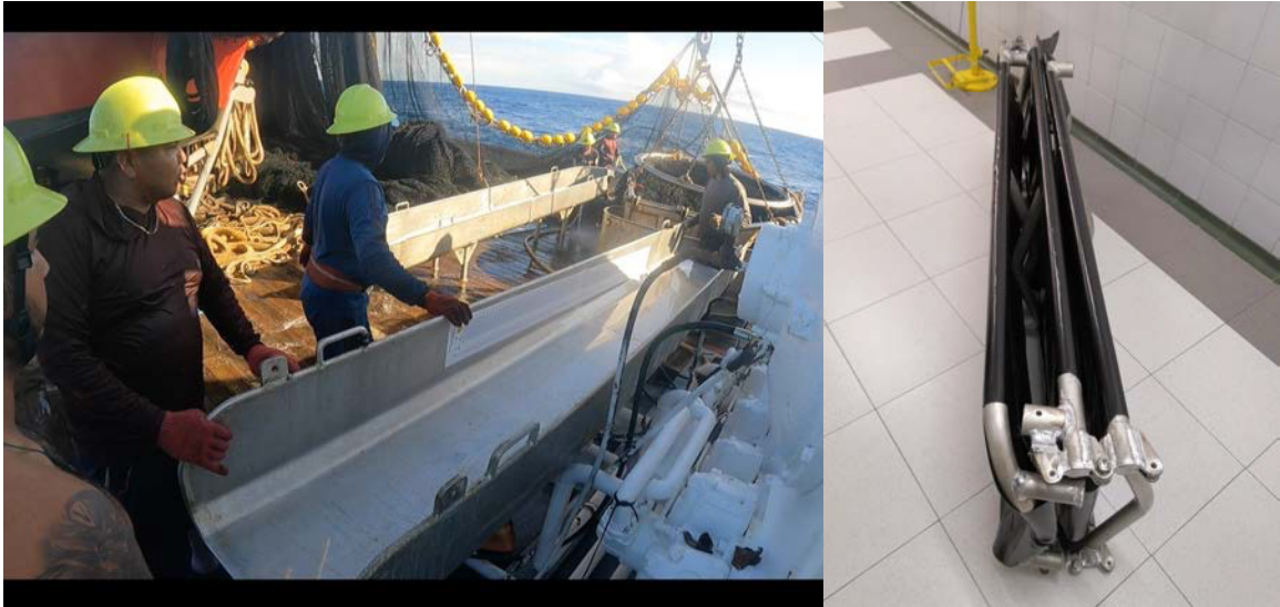
Figure 3. Detachable or foldable ramp systems, without or with a hopper, not permanently affixed, that can be quickly installed and removed during each fishing set. Photos: Cape Ferrat and ISSF (left), AZTI (right)
