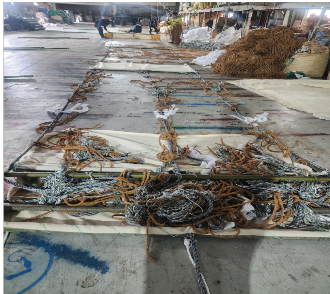
Figure 9. Bio-FAD used by Korean fleets, curtain-type dFAD made of bamboo, cotton rope, coir rope, and cotton canvas, with chain as weight.
