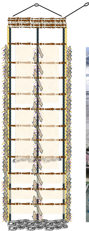
Figure 9. Bio-FAD used by Korean fleets, curtain-type dFAD made of bamboo, cotton rope, coir rope, and cotton canvas, with chain as weight.
